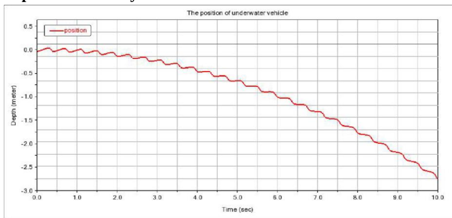
Figure 15: The change of the position of the center of mass in the first 10 seconds when harmonic motion.
