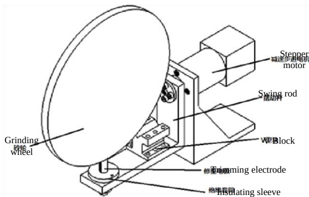
Figure. 2 Structure of the electric spark dressing device
